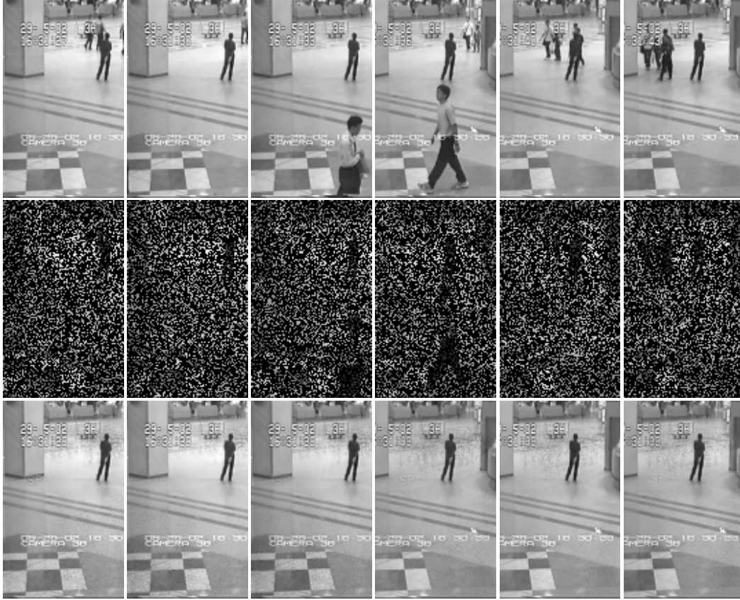
Figure 8. Background extraction using Geman. Samples from frame no. 40, 70, 100, 130, 170 and 200. Top row : Original images. Middle row : Training data with 70 % missing data. Bottom row : Reconstruction of background (bilinear method).
