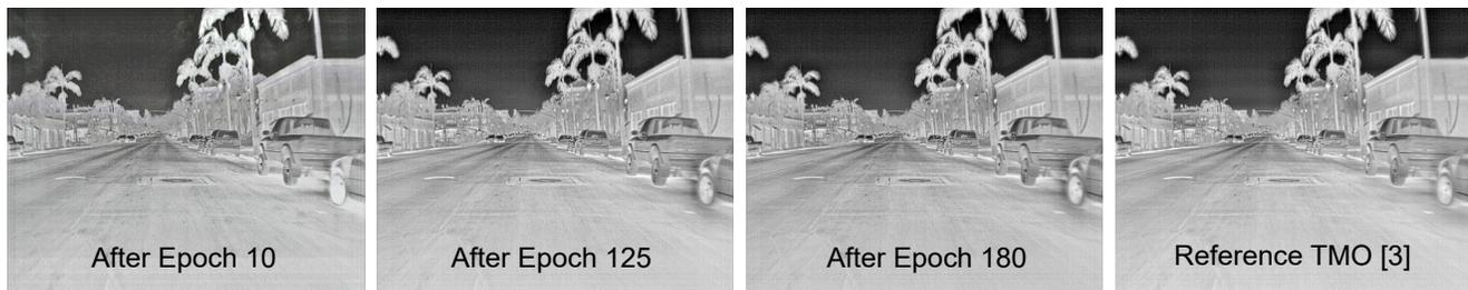
Figure 3. Evolution of the DCNN’s [2] TMO quality during transfer learning along the epochs. The clearly visible halos after epoch 10 disappear after epoch 125. However, noise is still more visible compared to the reference TMO. This gets better after epoch 180. Training is stopped after epoch 180.
