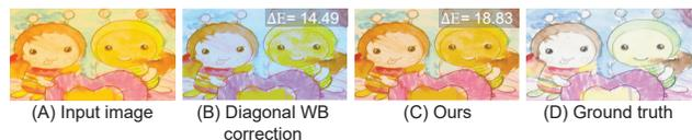
Figure 9. Failure example of the proposed method. (A) Input sRGB image. (B) Results using a diagonal white balance correction based on the *exact achromatic* reference obtained from the color chart. (C) Our result. (D) Ground truth image.
