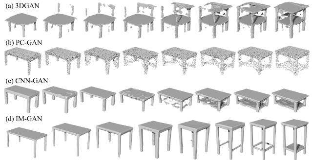
Figure 5: 3D shape interpolation results . 3DGAN, CNN-GAN, and IM-GAN are sampled at 64^3 resolution to show the smoothness of the surface is not just a matter of sampling resolution. Notice that the morphing sequence of IM-GAN not only consists of smooth part movements (legs, board), but also handles topology changes.
