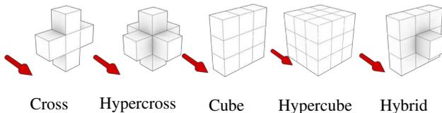
Figure 3: Various kernels in space-time. The red arrow indicates the temporal dimension and the other two axes are the spatial dimensions. The third spatial axis is hidden for visualization.
