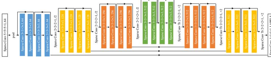
Figure 5: Architecture of MinkowskiUNet32.  $\times$  indicates a hypercubic kernel,  $+$  indicates a hypercross kernel. (best viewed on display) and the compatibility function in the CRF end-to-end.
