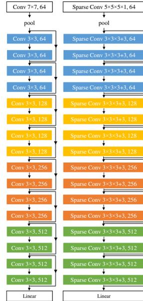
Figure 4: Architecture of ResNet18 (left) and MinkowskiNet18 (right). Note the structural similarity.  $\times$  indicates a hypercubic kernel,  $+$  indicates a hypercross kernel. (best viewed on display)
