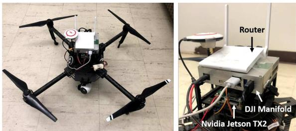
Figure 9. Left: top view of our prototype drone based on DJI Matrix 100. Right: the onboard processor module contains Nvidia Jetson TX2 and DJI Manifold. The communication between onboard systems and ground station is bridged by a router.
