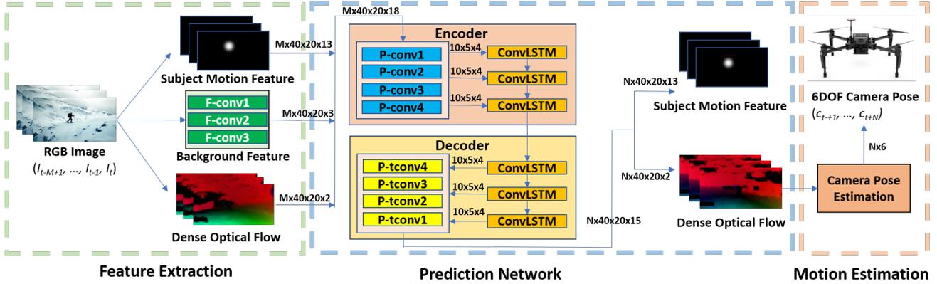
Figure 2. Overview of our imitation learning framework. The framework is consisted of three modules: 1) feature extraction, 2) prediction network and 3) camera motion estimation. We illustrate the dimension of the data flow as (time-step  $\times$  width  $\times$  height  $\times$  depth).
