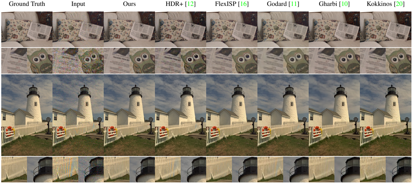
Figure 3: Burst demosaicking results on a real and a synthetic burst from the FlexISP dataset [16] (results are best seen magnified on a computer screen). Our model successfully restores the missing colors of the underlying images while suppressing noise. A PSNR comparison of the systems is provided in the supplementary material.
