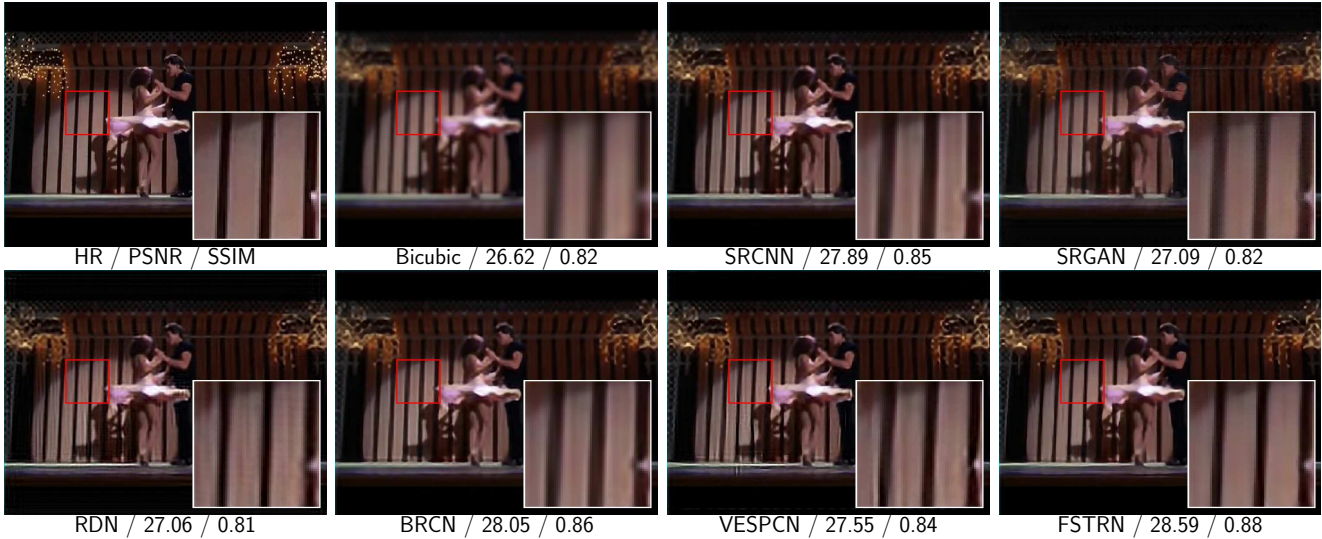
Figure 2: Visually observations on the original frames and the SR results on the Dancing video at \times 4 SR, it is noticeable that the proposed FSTRN approach not only achieves the highest PSNR and SSIM values, but also restores the finest texture with the fewest artifacts.
