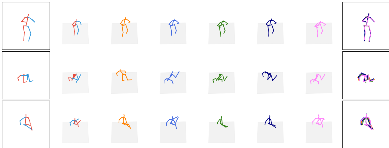
Figure 4: 3D Pose hypotheses generated by our network. The first column is the input of our network, i.e. the 2D joints estimated by the stacked hourglass network. The second column is the ground truth 3D pose, and the third to seventh columns are the hypotheses generated by our network. The last column is the 2D reprojections of all five hypotheses. The corresponding 2D projection and 3D pose are drawn in the same color. (Best view in color)
