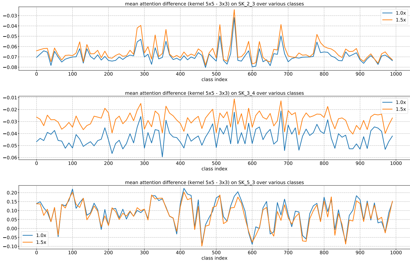
Figure 4. Average mean attention difference (mean attention value of kernel 5 \times 5 minus that of kernel 3 \times 3 ) on SK units of SKNet-50, for each of 1,000 categories using all validation samples on ImageNet. On low or middle level SK units (e.g., SK_2_3, SK_3_4), 5 \times 5 kernels are clearly imposed with more emphasis if the target object becomes larger ( 1.0x \rightarrow 1.5x ).
