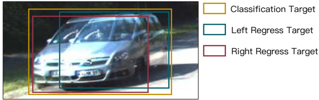
Figure 2. Different targets assignment for RPN classification and regression.
