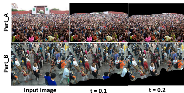
Figure 9. Illustration of the ROI regions extracted by different attention thresholds. The pixels which have the value of attention lower than t are changed to black.
