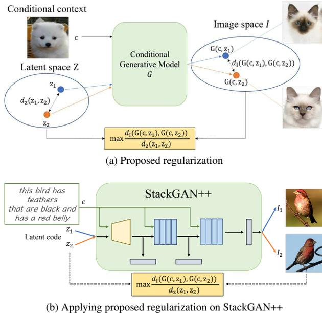
Figure 3: **Proposed regularization.** (a) We propose a regularization term that maximizes the ratio of the distance between generated images with respect to the distance between their corresponding input latent codes. (b) The proposed regularization method can be applied to arbitrary cGANs. Take StackGAN++ [29], a model for text-to-image synthesis, as an example, we easily apply the regularization term regardless of the complex tree-like structure of the original model.
