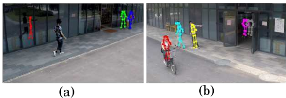
Figure 6. : Error mode examples. (a) Skeleton detection inaccuracy: bad detection of the person reflected in the glass lead to bad predictions by MPED-RNN. (b) Confusion in feature space: The person riding the bicycle (red) has a moving pattern “similar” to a person walking.
