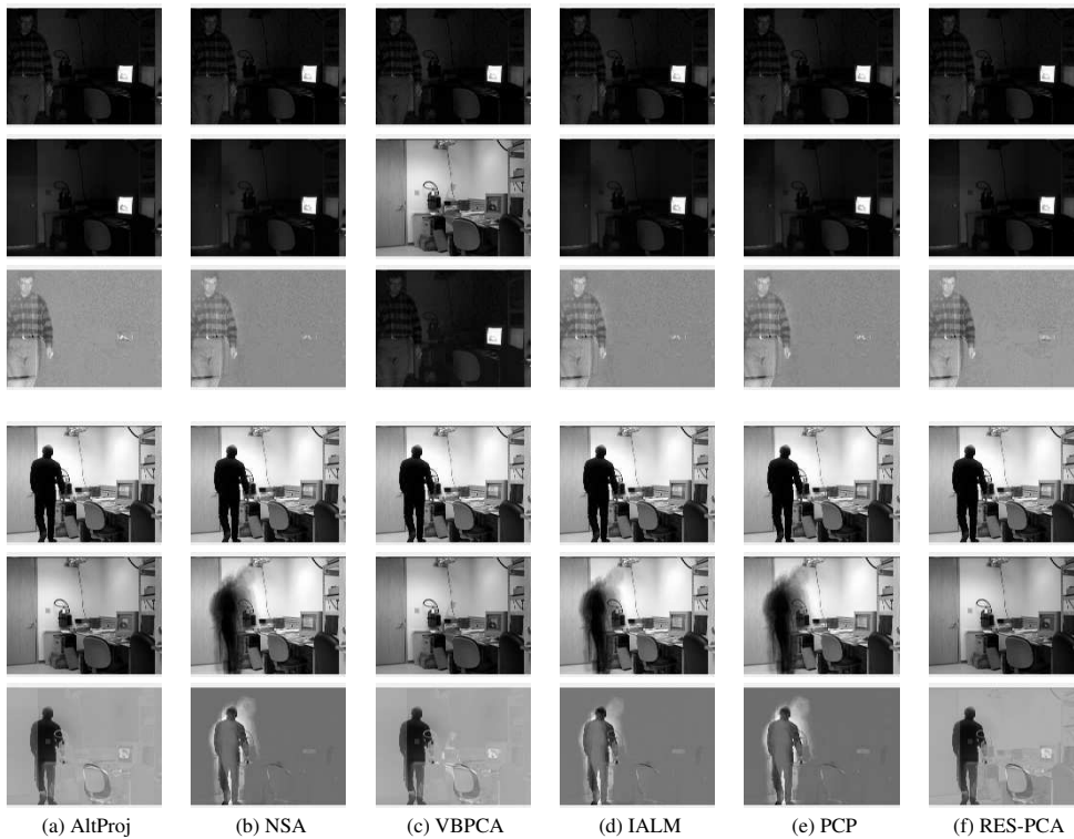
Figure 2. Foreground-background separation in the Light Switch-2 video. Within the first and last 3 lines, the top to bottom are the original frame, extracted background, and foreground, respectively.
