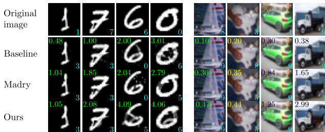
Figure 5: Adversarial examples with varied levels of noise \delta against three models: baseline, Madry defense [12] and our defense. Text on top-left of each image indicate \|\delta\|_2 ; text on bottom-right indicates the predicted class 4 .
