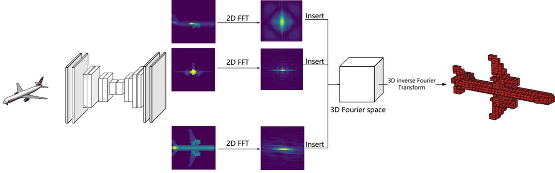
Figure 3. The pipeline of 3D reconstruction from images in the frequency domain. Taking an image as the input, we predict a series of thickness maps at different but specific projection views with a deep neural network. Each thickness map generates a 2D Fourier slice using the Fourier transform. All the 2D slices are inserted into a 3D Fourier space to constitute the Fourier transform of the 3D object. The 3D shape is reconstructed using the 3D inverse Fourier transform.
