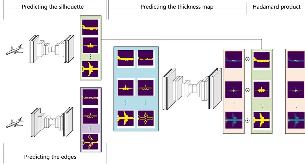
Figure 4. The architecture of the thickness map prediction network. Given an image, we predict a series of silhouettes and edges of the thickness map. All these silhouettes and edges are combined together to predict the thickness map.
