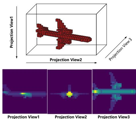
Figure 2. Example of thickness maps. We show three thickness maps of the 3D airplane model. The projection view is shown at the top. Each projection view is along a different axis of the Cartesian coordinate. The corresponding thickness map is shown at the bottom. The more lightened pixel means a more volumetric grid of the 3D shape belongs to the ray paralleling to the corresponding projection view.
