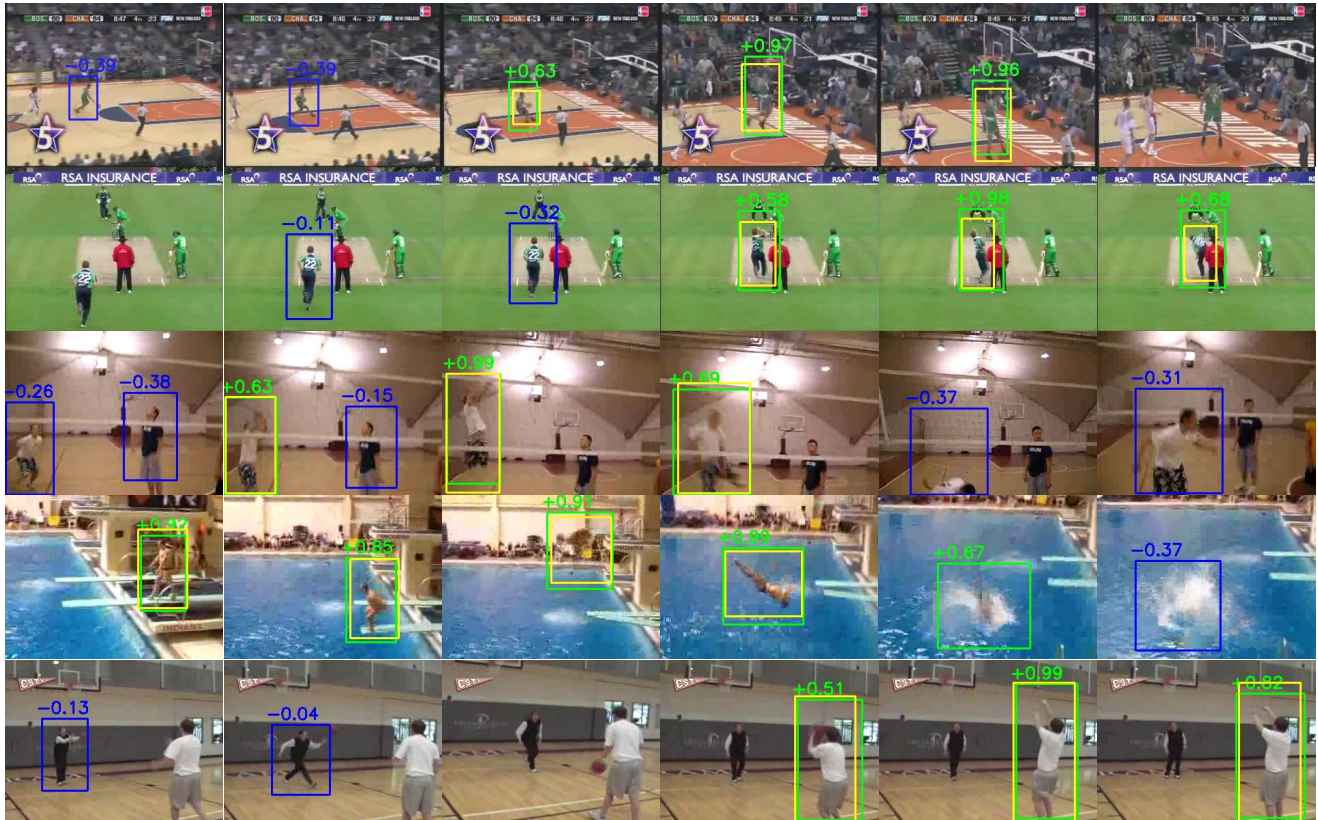
Figure 5. Predicted results of the proposed TACNet in four states: (a) Background (w/o box), (b) Transitional state (blue box), (c) Active state (green box) and (d) Ground-truth (yellow box).
