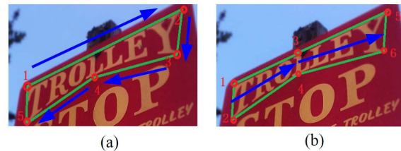
Figure 2. Two methods for adaptive text region representation. (a) text region represented by corner points; (b) text region represented by pairwise points on its top and down boundaries.
