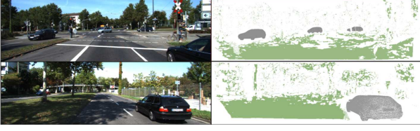
Figure 4. Left column: left target images ( L_t ). Right column: the regions selected in the RDVO module (i.e., region \mathcal{S} described in Eq. (5)) in green overlaying on the ground truth moving object mask in grey.
