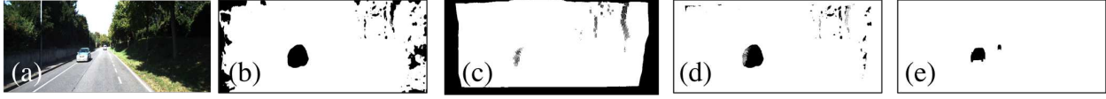
Figure 3. An example of our rigid potential. (a) Image. (b) Flow consistency map. (c) Visibility mask \mathbf{V}_f . (d) Rigid potential. (e) Ground truth rigid mask. We can see flow consistency falsely indicates rigid potential in occluded regions.
