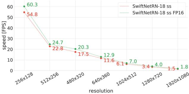
Figure 1. Comparison of inference speeds on the Jetson TX2. The same model, ResNet-18 single scale model, was ran using 32 and 16 bit floating point precision.
