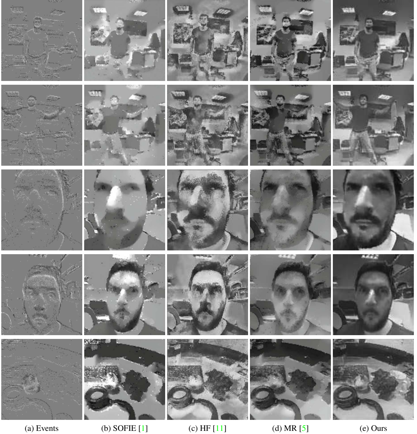
Figure 7. Qualitative comparison of our reconstruction method with various competing approaches. We used the datasets from [1]. The dataset does not contain ground truth images, thus only a qualitative comparison is possible. For SOFIE and MR, we used images provided by the authors, for which the parameters were tuned for each dataset. For HF, we ran the code provided by the authors, manually tuned the parameters on these datasets to achieve the best visual quality, and additionally applied a bilateral filter to clean the high frequency noise present in the original reconstructions.
