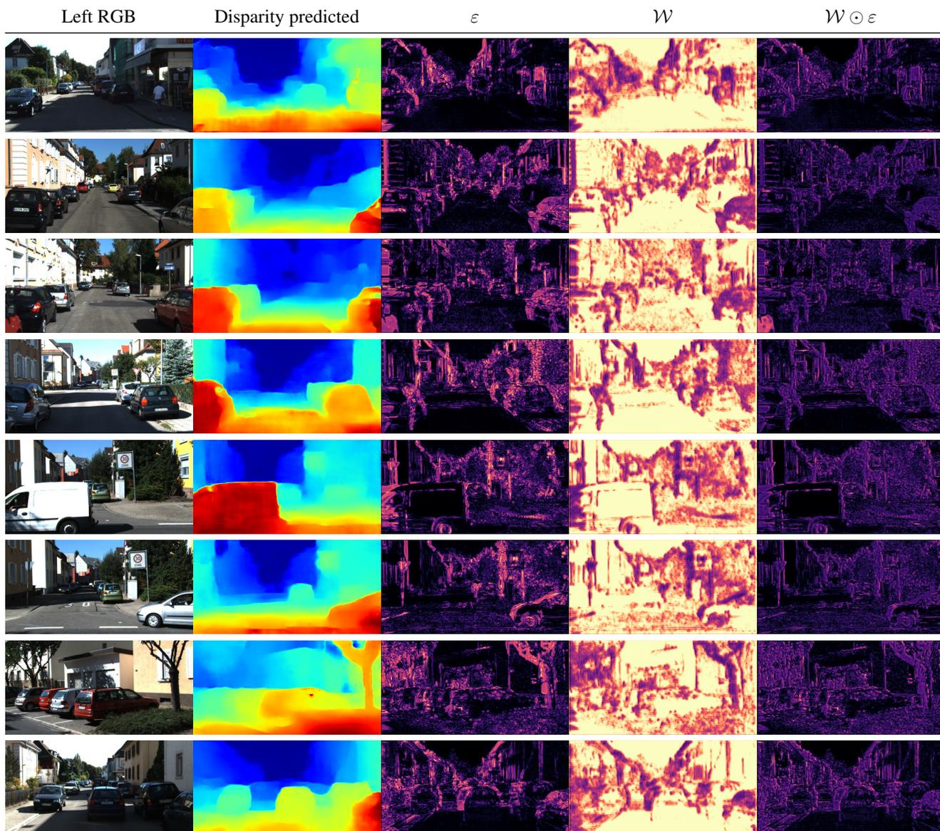
Figure 6. Visualization of our confidence estimations. From left to right: left rgb frame from a stereo pair, disparity predicted by Dispnet, reprojection error obtained as described in [Sec. 1.1](#), confidence mask predicted by our network, weighted re-projection error used for online adaptation. On the last three columns bright colors indicate high values.
