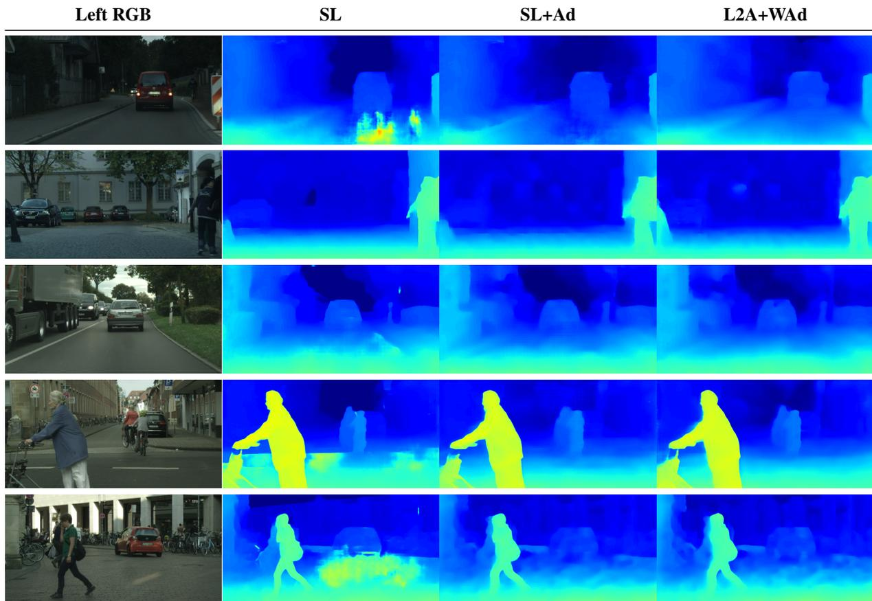
Figure 7. Qualitative results on the Cityscapes dataset. From left to right: left rgb frame from a stereo pair, disparities predicted by DispNet using as method **SL**, **SL+Ad** and **L2A+WAd** respectively. On the last three columns bright colors marks high disparity values. The number of adaptation steps performed increase together with the rows.
