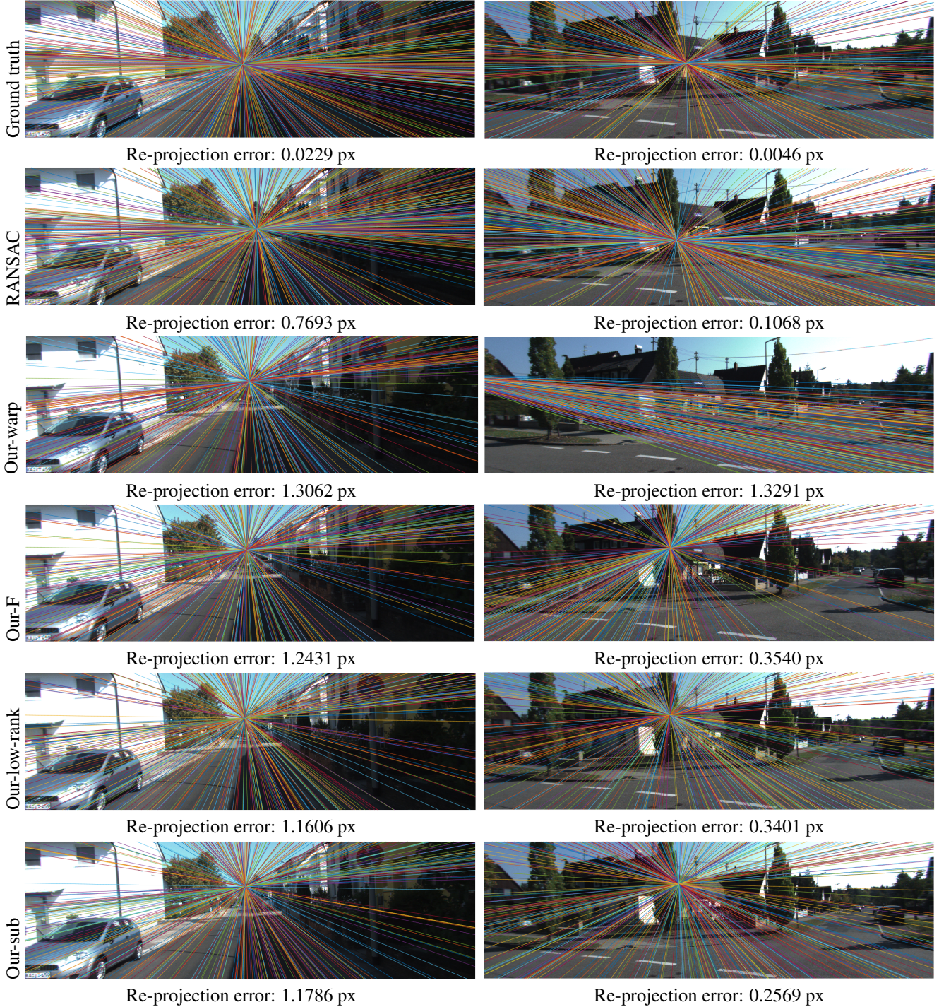
Figure 1. Epipolar lines of a random subset of inliers. We randomly select 300 points from ground truth flow as a subset of inliers and visualize their epipolar lines. The ground truth \mathbf{F} is computed from ground truth flow. The RANSAC represents the \mathbf{F} that computed from normalized eight point algorithm with RANSAC (for 5000 iterations). We illustrate our \mathbf{F} estimations of each method using Our-warp, Our-F, Our-low-rank and Our-sub. The camera in the left scene moves forward while the right one turns sharply.
