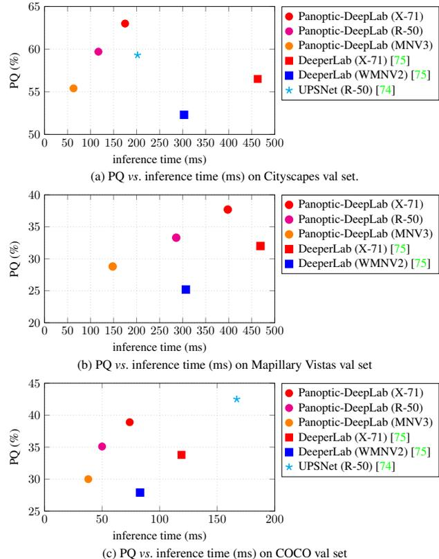
Figure 3. PQ vs. Seconds. Our Panoptic-DeepLab model variants attain a better speed/accuracy trade-off across challenging datasets. The inference time is measured *end-to-end* from input image to panoptic segmentation output. **X-71**: Xception-71. **R-50**: ResNet-50. **MNV3**: MobileNetV3. Data points from Tab. 9.
