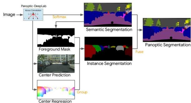
Figure 1. Our *Panoptic-DeepLab* predicts three outputs: semantic segmentation, instance center prediction and instance center regression. Class-agnostic instance segmentation, obtained by grouping predicted foreground pixels to their closest predicted instance centers, is then fused with semantic segmentation by majority-vote rule to generate final panoptic segmentation.
