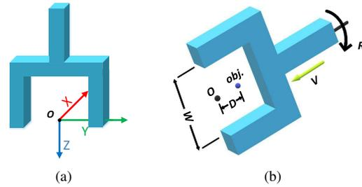
Figure 4. (a) The coordinate frame of the gripper. (b) Our new representation of grasp pose. “obj.” denotes object point. Our network needs to predict i) the approaching vector  $V$ , ii) the approaching distance from grasp point to the origin of gripper frame  $D$ , iii) the in-plane rotation around approaching axis  $R$  and iv) the gripper width  $W$ .
