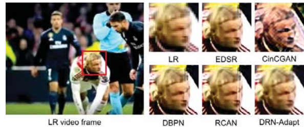
Figure 6. Visual comparison of model adaptation to real-world video frames (from YouTube) for 8\times SR.
