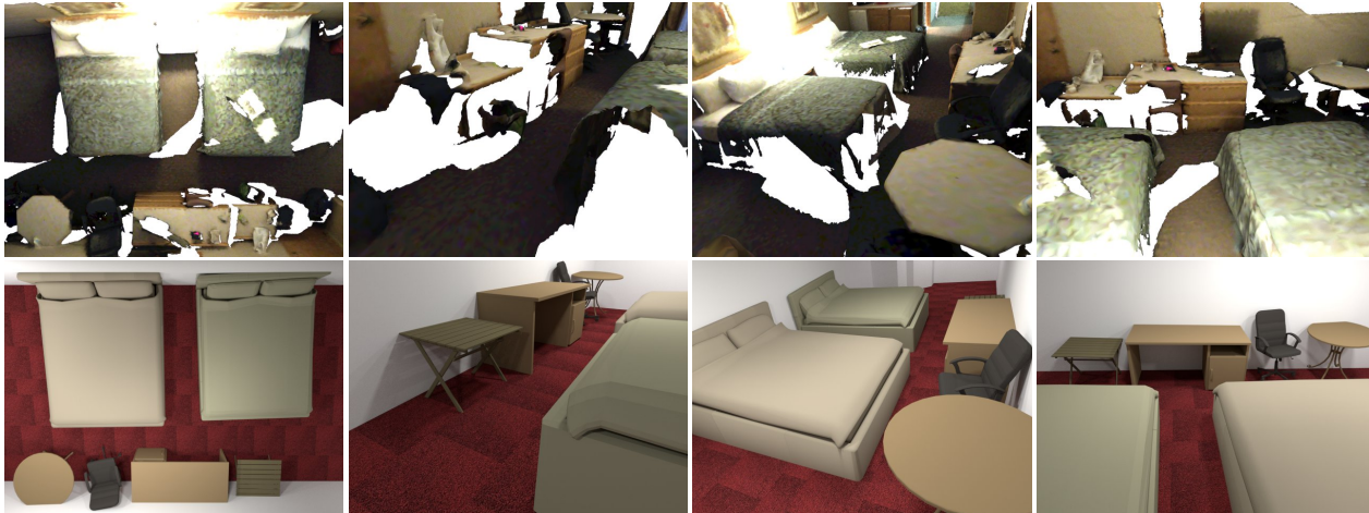
Figure 1. Given an RGBD sequence from a moving camera, we produce a 3D CAD recomposition of the scene. While a fused reconstruction (top) contains holes and noisy geometry, our recomposition (bottom) models the scene as a set of high quality 3D shapes from CAD databases.
