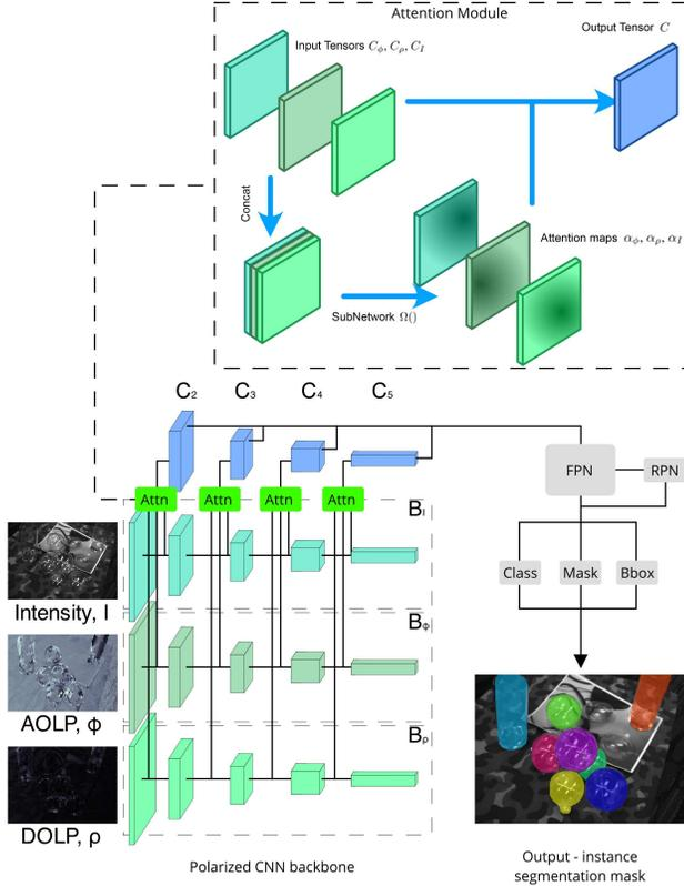
Figure 4: **Our Polarized CNN framework applied to Mask-RCNN.** We use three separate backbones and merge them with attention-fusion to produce high quality instance segmentation with Mask R-CNN. See Section 3.2.
