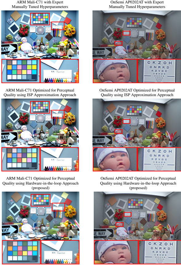
Figure 5: Optimization of ARM Mali-C71 and OnSemi AP0202AT ISPs for perceptual image quality.
