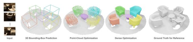
Figure 1: Given a localized input RGB sequence, FroDO dectects objects and infers their pose and a progressively fine grained and expressive object shape representation. Results on a real-world sequence from ScanNet [7].
