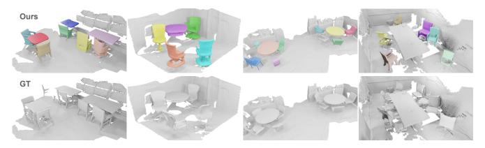
Figure 8: Qualitative results on four ScanNet RGB input sequences. We reconstruct multiple instances of the chair and table classes. While outputs are satisfactory for the first three scenes, the last one highlights failures due to heavy occlusions and partial observations. Top row: Object instances reconstructed by FroDO are shown in colour while grey shows the ground truth background (not reconstructed by our method) for reference. Bottom row: full ground truth scan for comparison.
