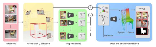
Figure 2: Given a sequence of calibrated, and localized RGB images, FroDO detects objects and infers their shape code and per-frame poses in a coarse-to-fine manner. We demonstrate FroDO on challenging sequences from real-world datasets that contain a single object (Redwood-OS) or multiple objects (ScanNet).
