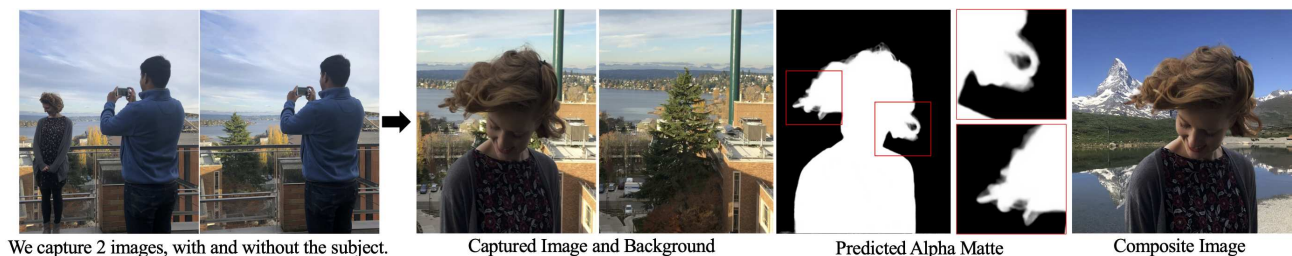
Figure 1: Using a handheld smartphone camera, we capture two images of a scene, one with the subject and one without. We employ a deep network with an adversarial loss to recover alpha matte and foreground color. We composite the result onto a novel background.
