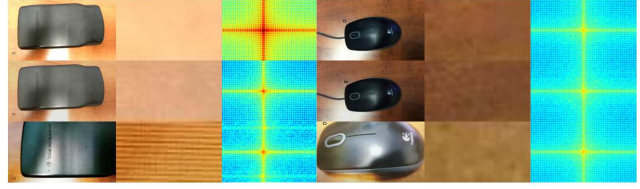
Figure 7. Visual comparison of live (first row), synthetic spoof (second row), and real spoof (third row) images. Columns are whole image, image patch, and the FFT power spectrum of the image patch. Each synthetic image was generated from a live image. The corresponding ground truth spoof images (third row) are collected with the target sensor/spoof medium combination.
