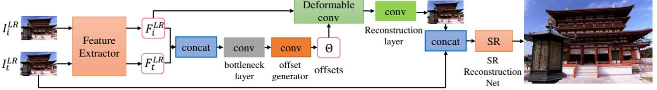
Figure 2. The proposed TDAN-based VSR framework. Here, we only show the framework with one supporting frame. In our implementation, 4 neighboring supporting frames are used for exploring more temporal information.
