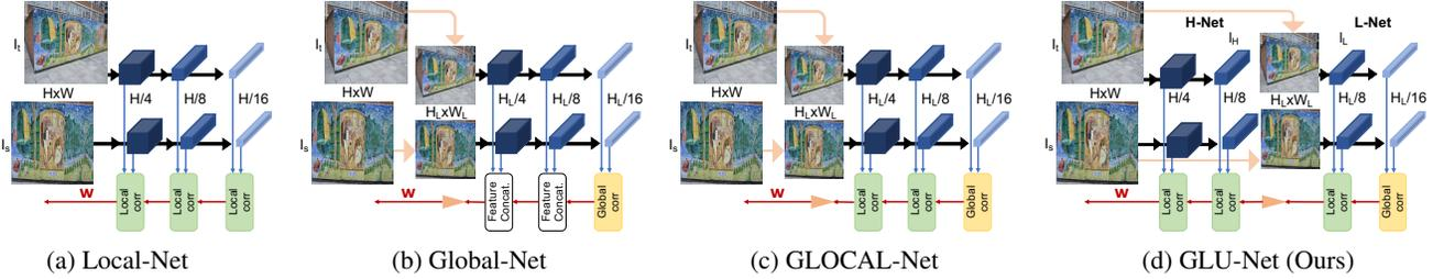
Figure 2. Schematic representation of different architectures for dense flow field estimation  $w$ . Local-Net (a) and Global-Net (b) employ *only* local and global correlation layers, respectively. Our GLOCAL-Net (c) combines both to effectively handle short and long-range displacements. GLU-Net (d) additionally employs our adaptive resolution strategy, thus capable of processing high-resolution images.
