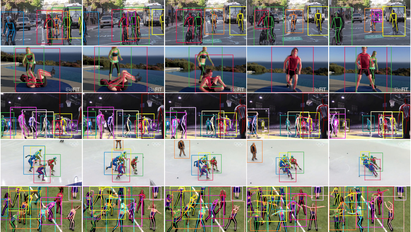
Figure 6: Visualization of the output of our approach on five videos from the PoseTrack dataset. Bounding boxes and poses are color coded using the track id predicted by our model. Solid bounding boxes indicate that the instance was localized by the person detector, while dotted bounding boxes were originally missed by the detector, but recovered by our approach.
