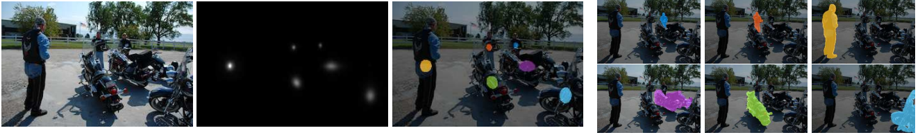
Figure 7: Illustration of instance mask inference in PCV. Left to right: input image, voting heatmap, detected peak regions (random colors assigned to each peak); six masks resulting from backprojection from color-matching regions.
