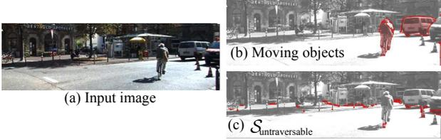
Figure 4. **Moving object and depth masking:** For a training image (a), our moving object mask (b) identifies pixels associated with moving objects. The set of pixels  $\mathcal{S}_{\text{untraversable}}$  (c) uses the training depth image to capture the footprints of small and thin objects.
