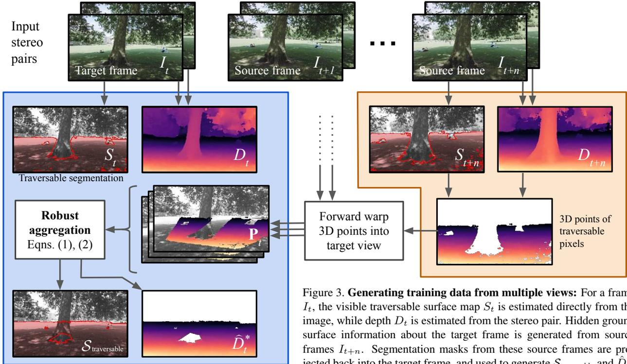
Figure 3. **Generating training data from multiple views:** For a frame  $I_t$ , the visible traversable surface map  $S_t$  is estimated directly from the image, while depth  $D_t$  is estimated from the stereo pair. Hidden ground surface information about the target frame is generated from source frames  $I_{t+n}$ . Segmentation masks from these source frames are projected back into the target frame, and used to generate  $S_{\text{traversable}}$  and  $\hat{D}_t^*$ .
