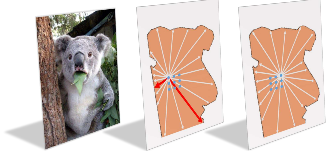
Figure 4 – Polar Centerness. Polar Centerness is used to down-weight such regression tasks as the high diversity of rays' lengths as shown in red lines in the middle plot. These examples are always hard to optimize and produce low-quality masks. During inference, the polar centerness predicted by the network is multiplied to the classification score, thus can down-weight the low-quality masks.
