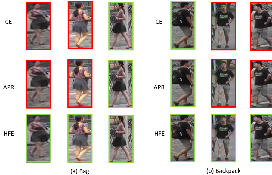
Figure 3. Visualization of recognition results. Correct predictions are bounded by green box and red box otherwise. (a) and (b) are prediction results of two IDs on bag and backpack respectively, each compared by three methods.
