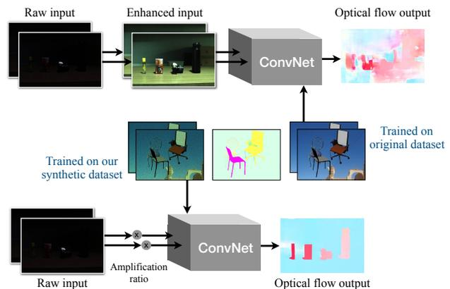
Figure 3. Above: two-step pipeline using existing methods for optical flow in the dark. Below: our pipeline for optical flow in the dark.
