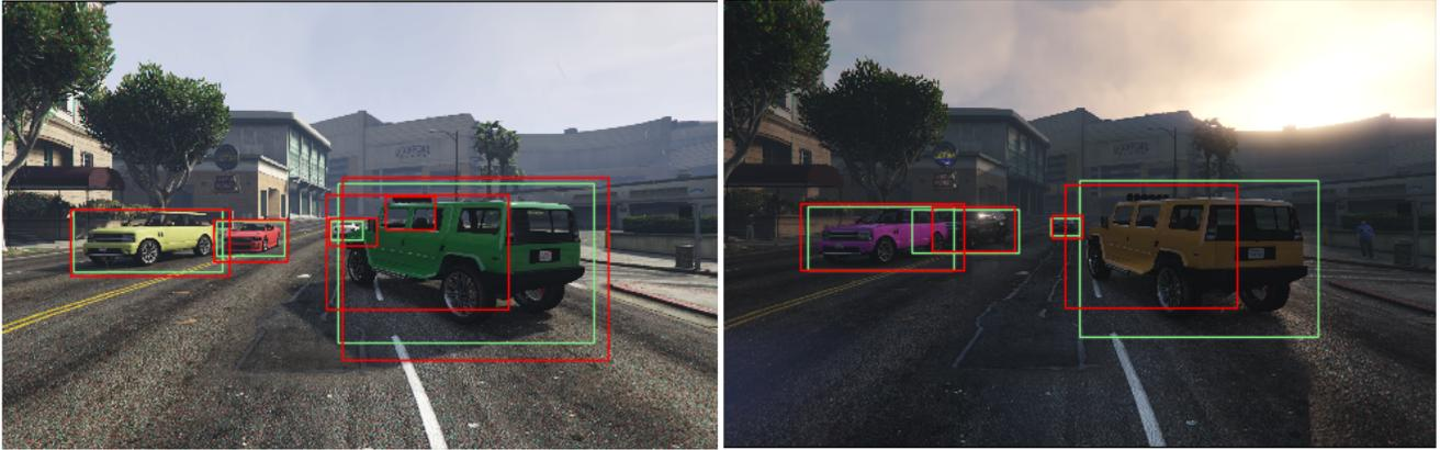
Figure 14: Failure images generated with Failure SCENIC Scenario 4 as shown in Figure 10 (b), with ground truth bounding boxes marked in green and prediction bounding boxes in red
