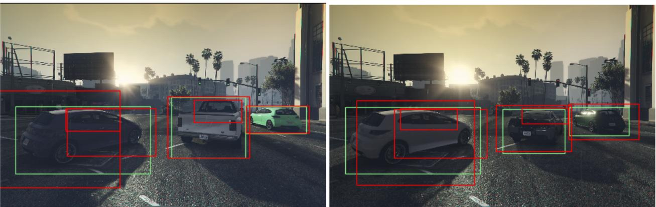
Figure 13: Failure images generated with Failure SCENIC Scenario 3 as shown in Figure 9 (b), with ground truth bounding boxes marked in green and prediction bounding boxes in red
