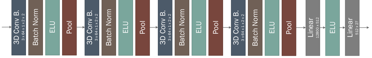
Figure 5: Architecture of our 3D convolutional network. We employed the same architecture for both our baseline and our approach, where the only difference is the 3D convolutional block used (3D Conv B): for the baseline a regular 3D conv, and for our method, our proposed HO-CP conv-S. Each convolution is followed by a batch-normalisation, non-linearity (ELU) and a max pooling (over 2 \times 2 \times 2 non-overlapping regions).
