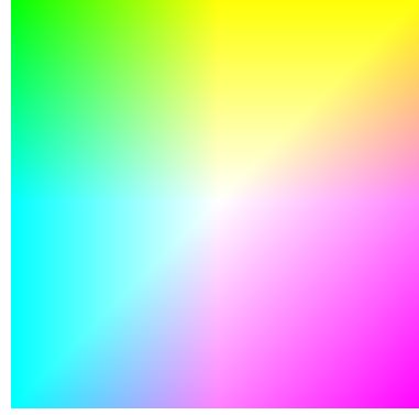
Figure 1. 2D color map used to encode the 2D flow. The white central pixel indicates no motion, while every other pixel's color encodes the vectorial displacement with respect to the central pixel.
