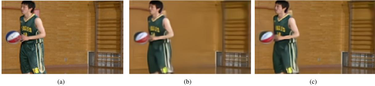
Figure 4. Visualized results of compressing the BasketballPass sequence. (a) The original frame  $x_9$ . (b) The predicted frame  $\bar{x}_9$  obtained by Add MVRRefine-Net model with  $\lambda = 64$ . (c) The predicted frame  $\bar{x}_9$  obtained by Add MMC-Net model with  $\lambda = 64$ . There are much more details in (c) than (b).
