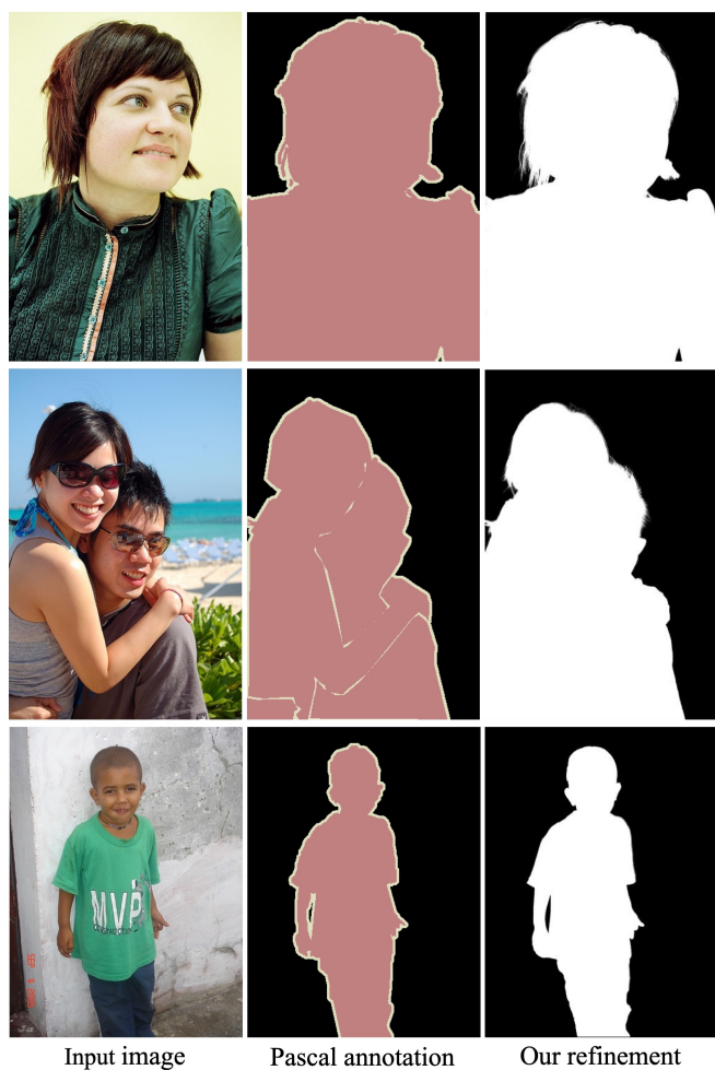
Figure 4: Using the proposed method to refine coarse human mask from COCO [5] dataset annotations, Pascal [3] dataset annotations and DeepLab [1] output (Best viewed in PDF with zoom).
