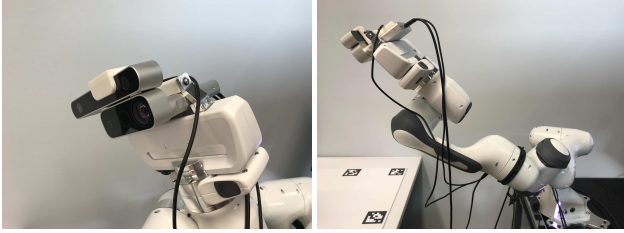
Figure 3: Robot configuration. Left: we mount both ZED stereo camera (top) and Microsoft Azure Kinect camera (bottom) on the end-effector of the robot, with a plastic fixture produced by 3D printing. Right: Franka Panda arm used to capture data.
