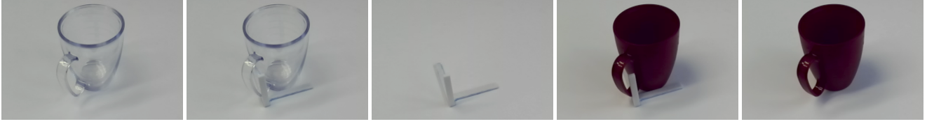
Figure 2: Illustration of our method of using marker to replace the transparent objects with its opaque twin. The white plastic marker was produced by 3D printing.
