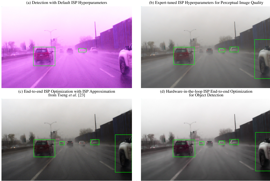
Figure 7: ARM MALI-C71 ISP for 2D automotive object detection example in rainy condition.
