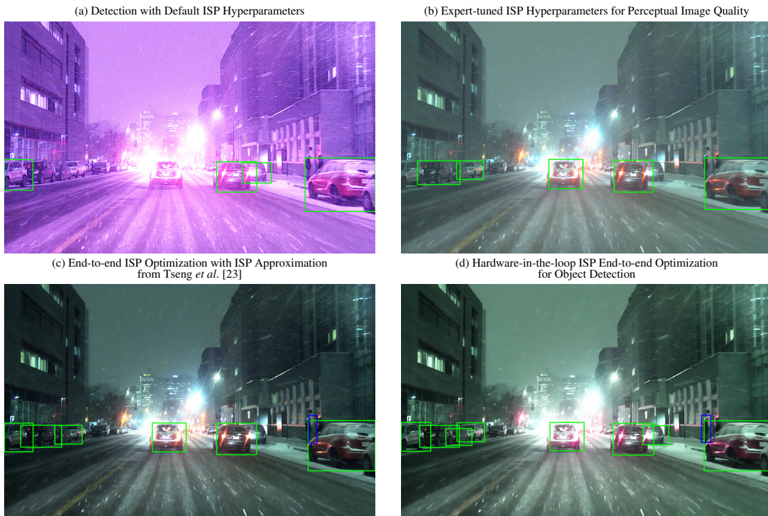
Figure 8: ARM MALI-C71 ISP for 2D automotive object detection example in night snowfall conditions.
