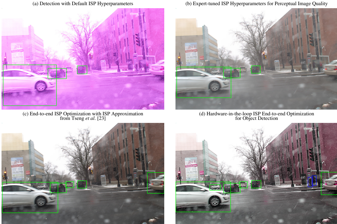
Figure 6: ARM MALI-C71 ISP for 2D automotive object detection example in snowfall condition.
