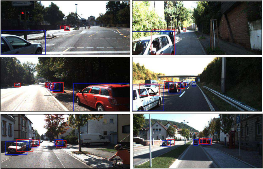
Fig. 5. Virtual KITTI examples are in the left column, GTA examples are in the right column. Blue boxes show correct detections; red boxes show detections missed by the FasterRCNN network trained on baseline, unaugmented image datasets but detected by FasterRCNNs trained on data augmented using our proposed approach for sensor-based image augmentation.
