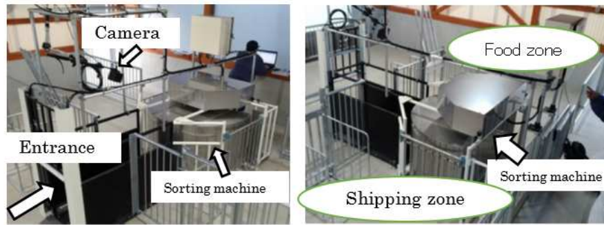
Fig. 2. Photograph of the pig sorting system (2018). A computer is placed outside of the pig room, and the system is controlled by a LAN connection. A Gig-Ethernet camera system is placed at the top of the system and observes the movement of the pigs.
